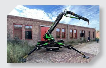
Another application of the Mini Crane is moving loads over short distances. The crane is easy to move and can move heavy loads over obstacles and through narrow passages. This makes it ideal for moving materials on construction sites or loading and unloading trucks in tight loading and unloading areas.
